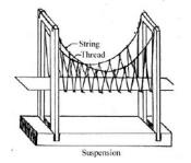
To build the bridges, use construction paper or poster board strips. Use building blocks, bricks or whatever for supports. Use toothpicks and thread for suspension bridge. Using toys cars, pile them on the bridge until they collapse. The boys love to try to bring about the demise of a bridge and are astonished at the strength of the truss and suspension bridges.
