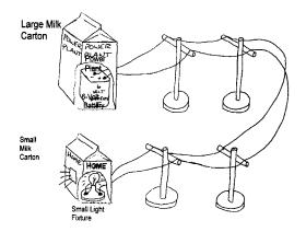
Make a small scale electrical system Equipment: 6 Volt Battery Insulated wire Small Light fixture
